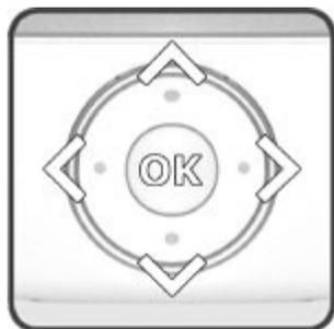
The navigation control is a 4 way control button (left, right, up, down) plus a central validation key. The navigation button is used to turn pages (right, left) to move a selection on the screen (up, down, right, left) and to validate a selection or call a contextual menu. Most of the actions can be done with this navigation button.
