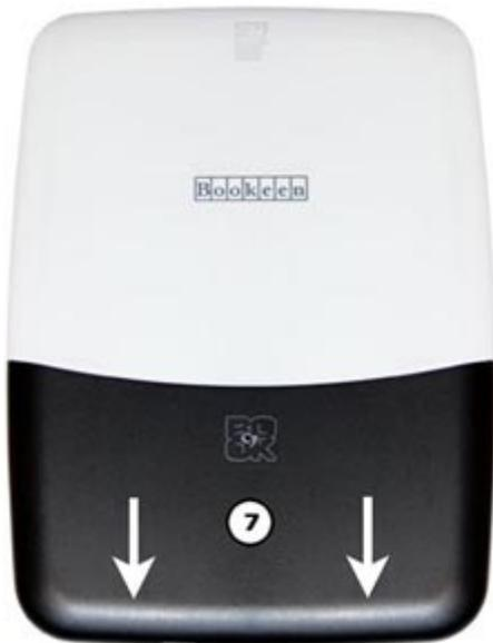
[7] Removable sliding plate: this plate can be easily slid to give access to battery and reset hole.
