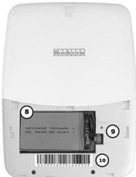
[8] Battery Compartment: Contains the Li-Polymer battery of the Cybook Opus.
