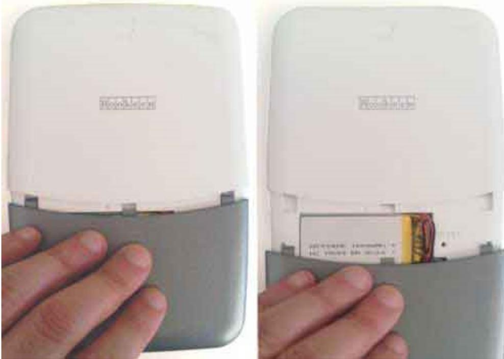
You can easily access the battery and the reset hole of your Cybook Opus. The battery and the reset hole are located in the back of the unit behind a removable sliding part of the external housing. No screws are needed to access this compartment.
